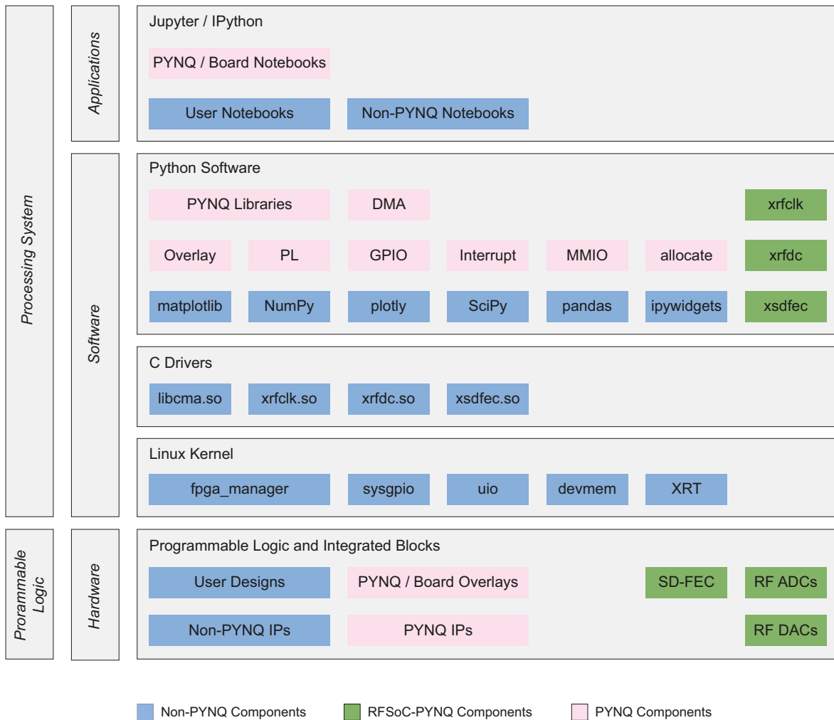
Figure A.2: Simplified diagram of the PYNQ framework and ecosystem (contains relevant RFSoc software libraries).
