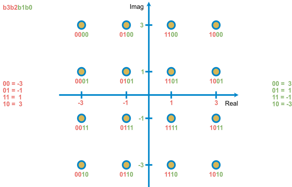
Figure 15.9: Gray coded symbol mapping for 16-QAM.
