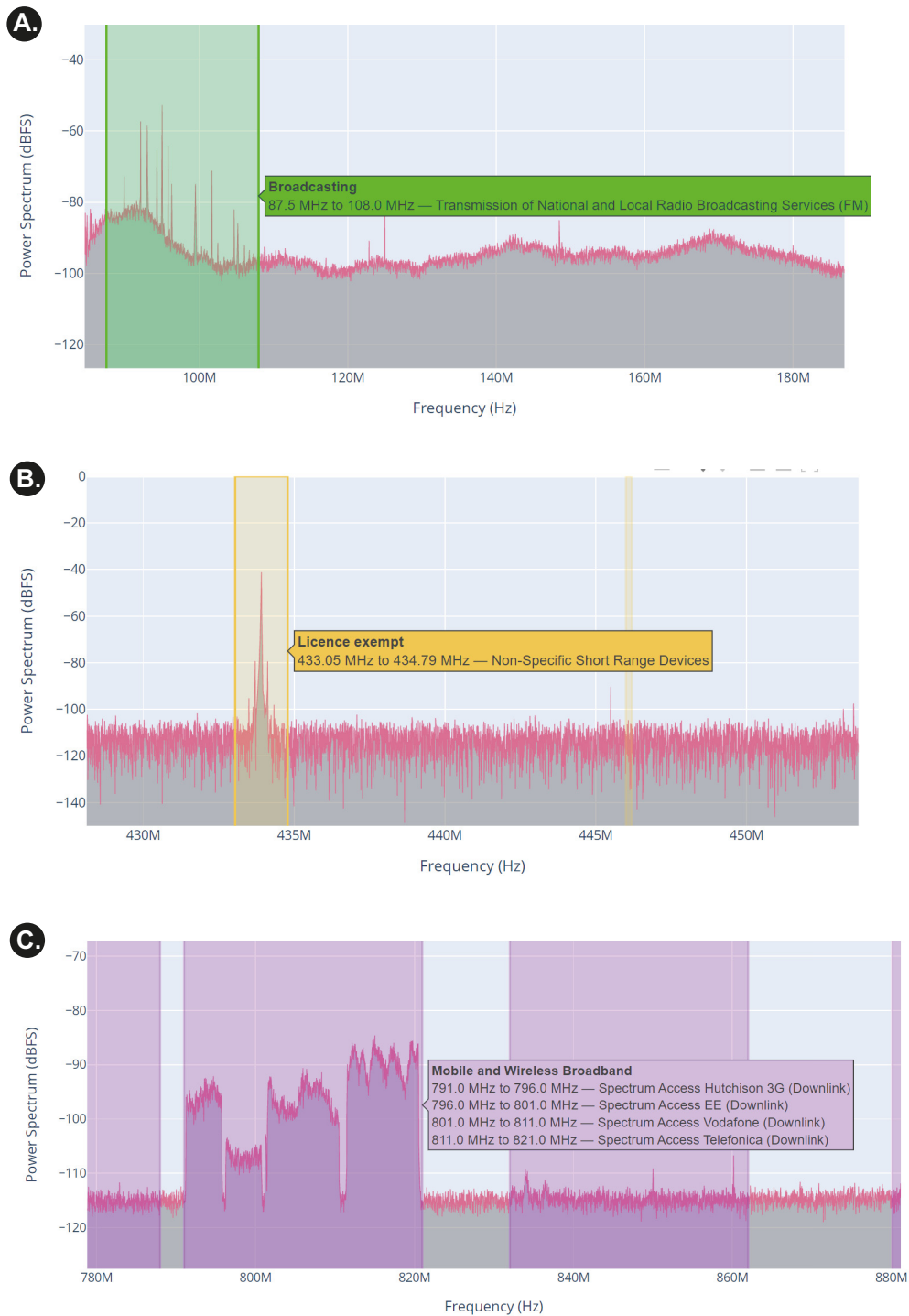
Figure C.1: Screenshot A: viewing the FM radio spectrum; Screenshot B: spectrum of a licence-exempt band (UK only); Screenshot C: spectrum from the mobile and wireless broadband sector.
